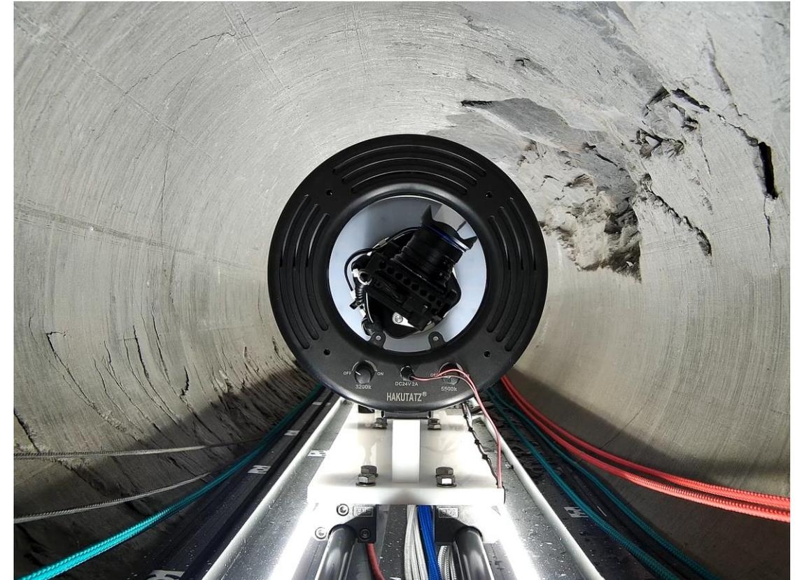
Semiautomatic recording of borehole breakouts with 0.2 mm resolution from 3-D photogrammetry
